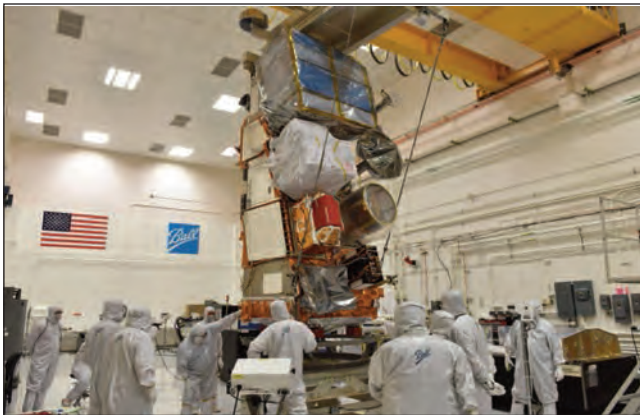
JPSS-1 spacecraft and United Launch Alliance Delta II payload attach fitting finish fit check.
