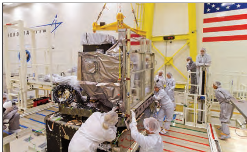
The GOES-R Advanced Baseline Imager (ABI) is installed onto the GOES-R spacecraft at Lockheed Martin in Littleton, Colorado, on October 13, 2014.
