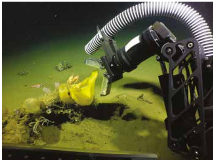
Remotely operated vehicle Yogi collects a sponge sample for taxonomic identification and habitat characterization. Credit: NOAA and the Global Foundation for Ocean Exploration.
